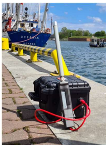
Self-powered mobile devices with directional and omnidirectional antennas
