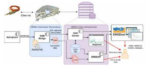
Figure 1: OBSEA's real-time underwater noise monitoring system dataflow
