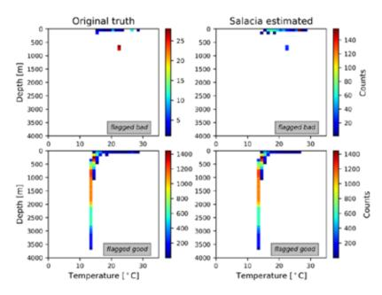
Figure 1: Temperature / Depth plots for truth (left) vs. Salacia (right). Salacia predicted with accuracy larger than 90 % for both good (green) and bad (red) flags.
