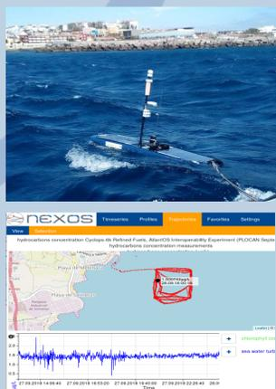
Within the **NeXOS project** two PUCK-enabled sensors (Mini.1 Hydrocarbons detector and Smart Hydrophone A1) were deployed in a SeaExplorer glider at Runde Island, Norway (September 2017). The SWE Bridge was integrated within the glider controller. The acquired data was transmitted in near real-time using an Iridium link to a SOS server.
