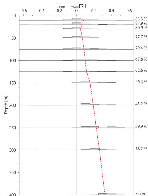
Histogram of temperature differences between visual reading ( $T_{JODC}$ ) and traced ( $T_{traced}$ ) at standard depths. Red line shows mean difference and axis label at right shows the ratio within  $\pm 0.1$  degree Celsius. Note that JODC (Japan Oceanographic Data Center) means visual reading temperature data are stored in JODC.
