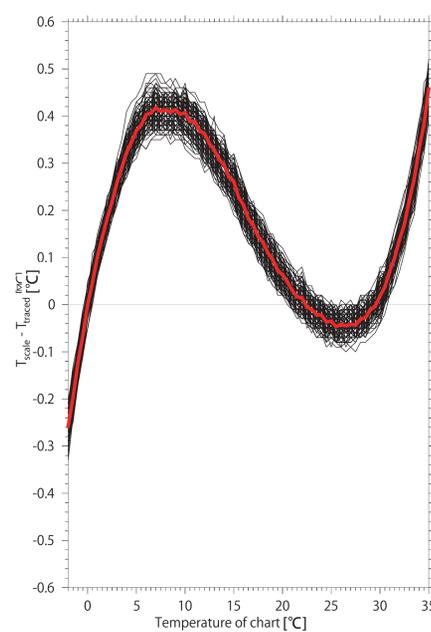
Temperature differences between horizontal scale of strip chart ( $T_{scale}$ ) and traced horizontal axis ( $T_{traced}$ ) for 100 strip charts (black lines) and mean difference (red line).
