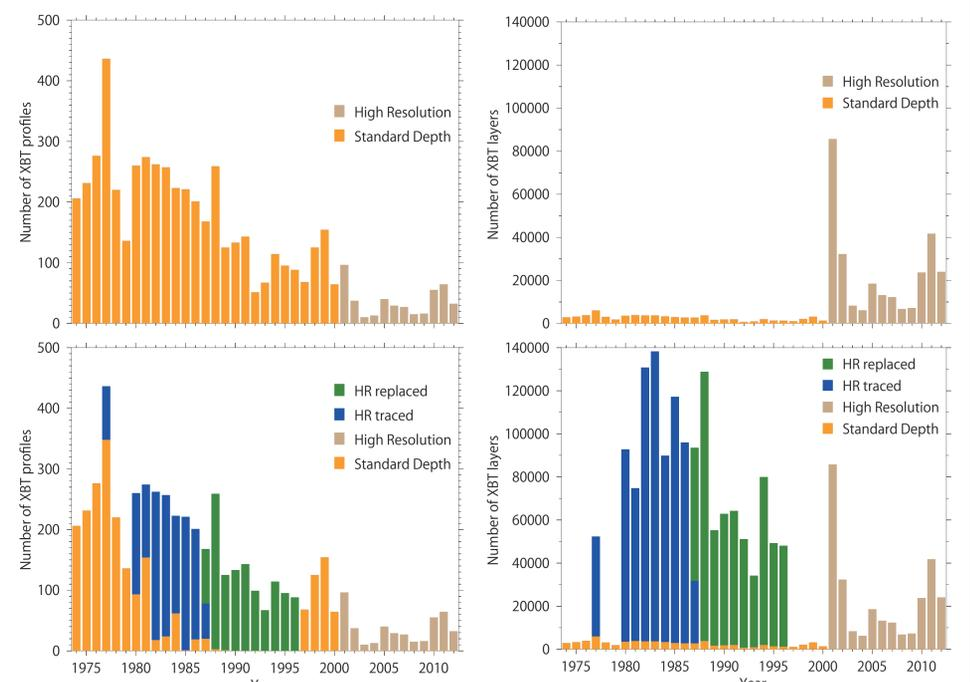
Annual changes of the number of XBT profiles (left panels) and XBT layers (right panels) by R/V Ryofu-Maru. Upper panels shows existing database of JODC and lower panels show the new one in this study. Blue indicates traced data and green indicates replaced with high resolution data by digital converter which were found by this study.
