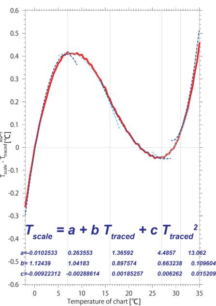
Quadratic functions (blue lines) to mean temperature difference curve fitting (red line) in each five temperature domain [ $< 7$  |  $7 - 16$  |  $16 - 27$  |  $27 - 31$  |  $31 <$ ]
