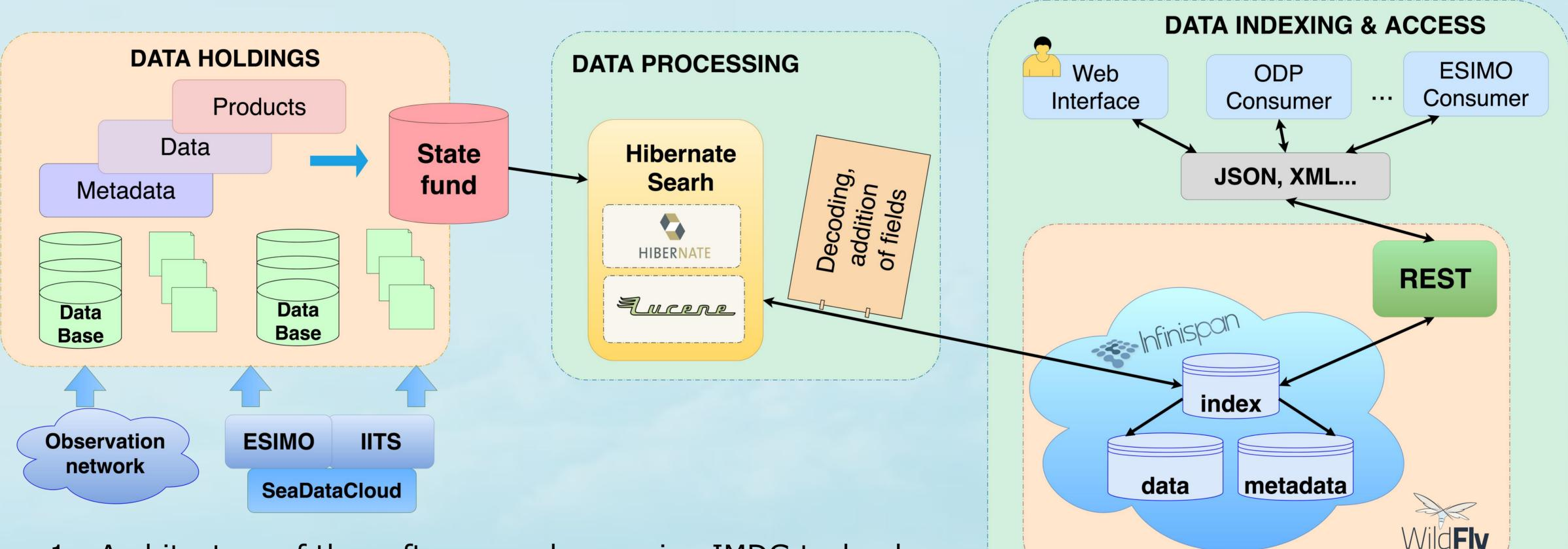
Figure 1 - Architecture of the software package using IMDG technology for storing, accessing and searching for information
